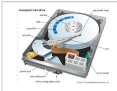
Computer Hard Drives were the Storage Device of choice for many years. These drives consist of rotating disks where the data is stored. These drives have a normal life expectancy of 3-5 years. Once they start to fail, your ability to recover the data can become difficult to recover or could be completely lost.
